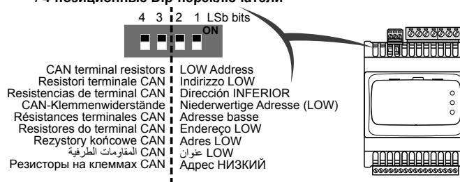
4 DipSwitches. Dip Switch 1-2. LSb bits. Refer to User Guide to configure address.
