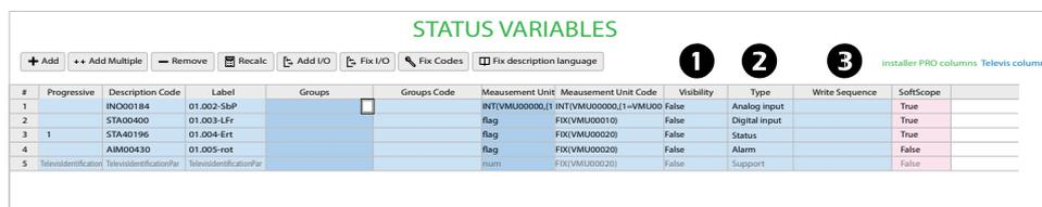
The **Fix Codes** button allows you to regenerate the description code of an inserted description if it is present in the Eliwell dictionary or in the custom dictionary (Custom Dictionaries, page 439).
