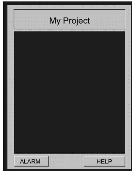
You can set these dimensions of the frames and insert some controls which are active whatever the currently loaded page. Consequently, frames are useful to host the objects which have to appear in the whole project. In this way you do not need to duplicate them in each page.
