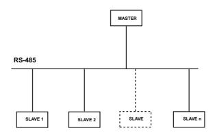
The type of connection, wiring, signal levels and communications parameters such as parity and baud rate are defined. Controllers can be connected directly over a network or via modem. Each device must be assigned a unique address for the entire network.
