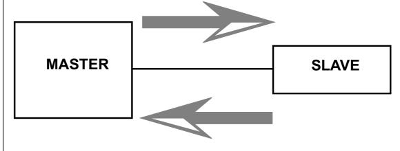
Generally speaking, the protocol describes the routines a device has to use to: request access to another device, respond to queries from other controllers or devices, detect and signal errors and, lastly, establish a common format for both content and layout in the various fields of the message.
